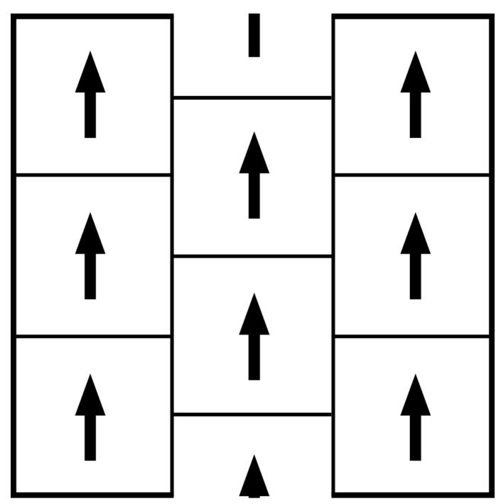
In this case, the tiles are installed in the same running direction but with a cross-joint pattern.
