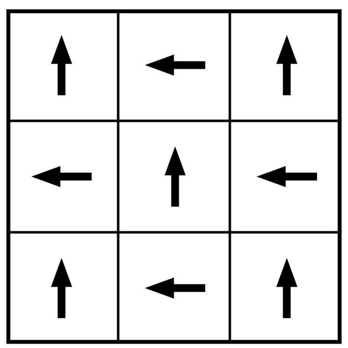
The tiles are laid with a half offset, following the same direction as the other row. This method eliminates cross joints.
